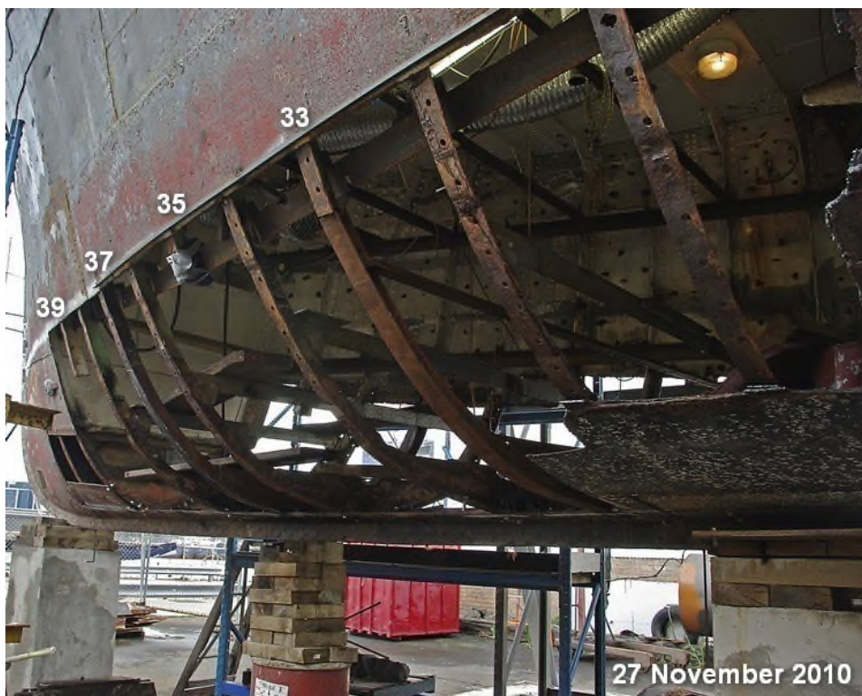
Removal of corroded plates and frames from the forward hull Jeff Malley
