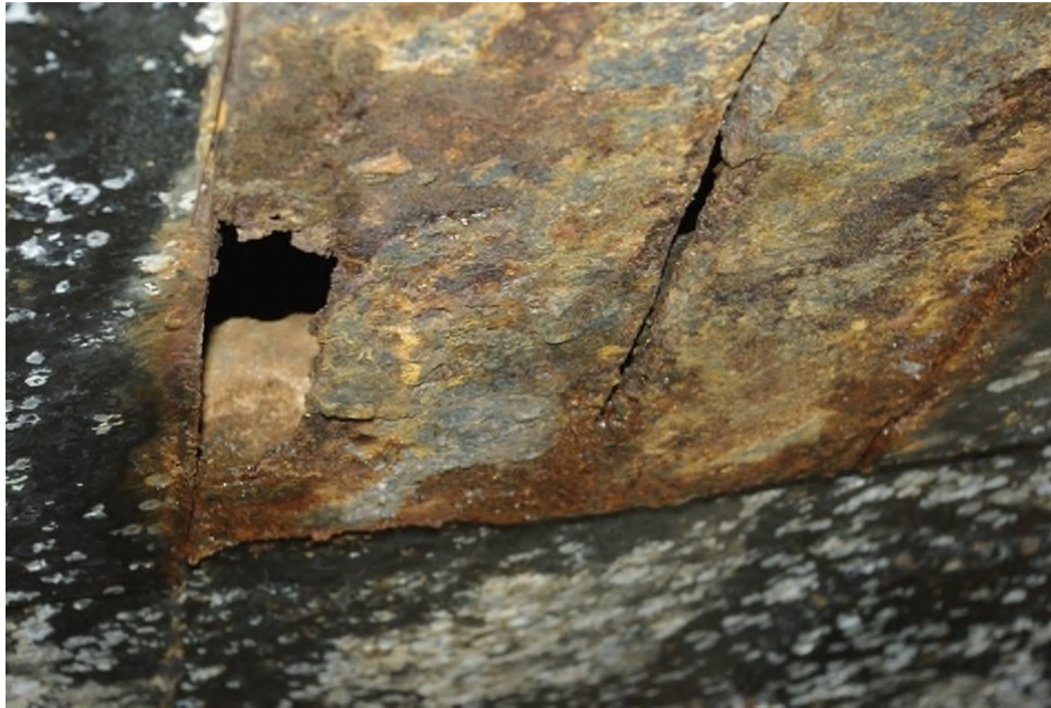
Plate corrosion on outside of hull under a "doubler". Jeff Malley
